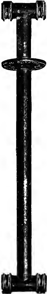
FIG. 126.—Attaching rod for suspending a switchboard operator's transmitter. It is secured to the top of the switchboard, as shown in Fig. 107, by the screw plate; the flexible conducting cords passing through the pulleys and being held back by pulley weights.
